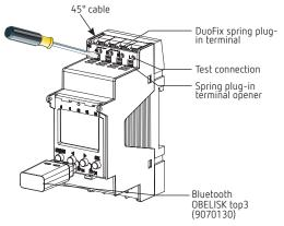
Check the depth of the control cabinet when OBELISK top3 is connected. The depth must be > 94 mm.
