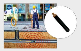
The MLS 55-3 pipeline transmitter sonde is a slim battery-powered mini-transmitter and has a range of 5 m. Attached to a drain rod, or fibreglass push rod cable, by one of the 3 adapters provided it is used to locate ductworks or blockages. A heavy duty protective cover is available.
