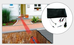
With the Easyloc house connection set, you can quickly and easily track the services leading from the house out to the main line. The set consists of connecting cables for standard 13A safety electricity sockets, cable TV and telephone sockets. To send a signal directly to the house connection the transmitter is connected to the relevant socket.
