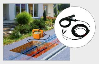
The Easyclamp transmitter clamp is used to transmit the Easyloc transmitter 33kHz signal onto and along live cables without shutting off the power to the cables. The Easy clamp is connected to the Easyloc Tx transmitter and installed around the cable to be traced and provides effective cable route tracing.
