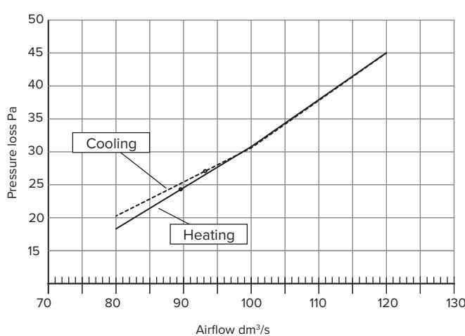
**Pressure loss of the fluid side**
