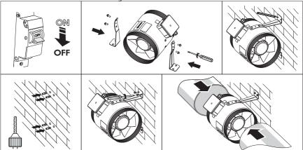
The VKOM fans are installed into air duct by means of an RM reducer which enables joining different diameter ducts. Once done, the assembly is secured with clamps. The VKOM delivery package includes mounting brackets for attaching the units to a wall. The power is supplied via the remote-position terminal box. VKOM fan installation:
