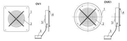
The VKF fans consist of a casing 1 with round flanges on both sides providing connection for a cross piece complete with an electric motor and impeller 4 made with bolts 3. The impeller rotation direction depends on the type of electric motor used. The electric motor casing has an M4 threaded hole and yellow-green cables for connection to the protective ground circuit.
