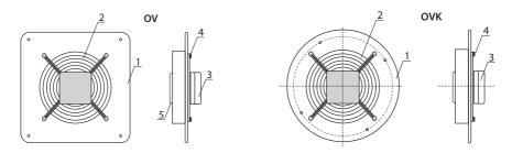
**The OV1 and OVK1 fans** consist of a casing 1 made of polymer-coated stainless steel with a square (OV1) or round (OVK1) flange providing connection for a grille 2 made with bolts 4. The motor and impeller 5 are mounted on a bracket inside the casing. OV1 and OVK1 fans are equipped with a terminal box with a cable for remote connection.
