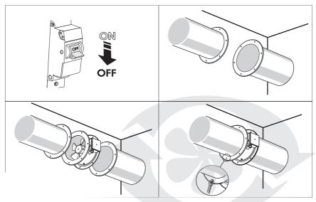
The OVP fans are installed into air ducts by means of clamps. The OVP delivery package includes mounting brackets for attaching the units to the ceiling or a wall. The power is supplied via an external terminal box mounted to the fan casing. OVP fan installation:
