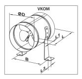
The VKOM fans are equipped with RM (polymer-coated steel) and RM  $\dots$  Zn (galvanised steel) reducers for connection to 150 mm, 200 mm and 250 mm air ducts. The reducers are not included in the delivery set and must be ordered separately.
