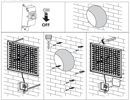
The VKF fans are installed into air ducts by means of connection flanges. The fans must be installed in such a way so that the direction of the arrow shown on the casing matches the direction of air flow in the system. The power is supplied via the remote-position terminal box. VKF fan installation:
