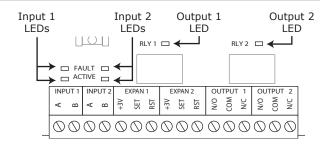
The device has six indication LEDs. They operate as follows:
