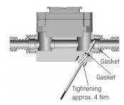
Straight inlet: MULTICAL® 402 requires neither straight inlet nor straight outlet to meet the Measuring Instruments Directive (MID) 2014/32/EU and EN 1434:2007. A straight inlet section will only be necessary in case of heavy flow disturbances before the meter. We recommend to follow the guidelines of CFN CR 13582
