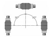
MULTICAL® 402 may be turned upwards to max. 45° and downwards to max. 90° compared to the pipe axis.
