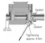
Possibly supplied glands can only be used for PN16. For PN25 installations shall be used suitable PN25 glands.
