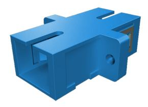
Our range of high quality SC adaptors have high precision alignment sleeves for reliability and improved reconnectability. For singlemode applications a ceramic sleeve is supplied to ensure a high precision alignment. For multimode applications a phosphor bronze sleeve is supplied. The housing is available in different colours with options for flange or flangeless body, metal clips or inbuilt clips.
