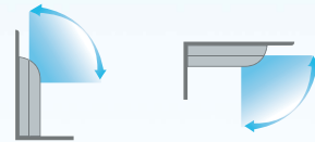
The unit can be installed either horizontally on the ceiling or vertically against the wall.
