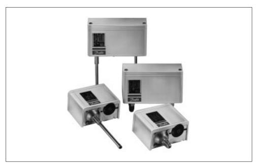
KP pressure controls are used as protection against too low a suction pressure or too high a discharge pressure on compressors in refrigeration and air conditioning plant. KP pressure controls are also used for starting and stopping refrigeration compressors and fans for air-cooled condensers.
