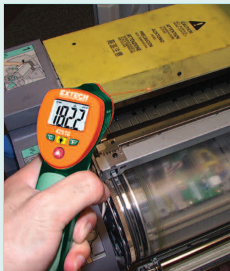
Electrical Troubleshooting for hot spot detection
