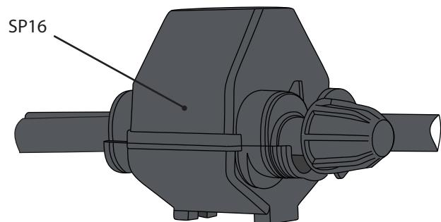
SP16 connector cover is not included with insulation piercing connector SLW25.2 package.
