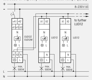
Maximal capacity of each additional lamp 500 W.
