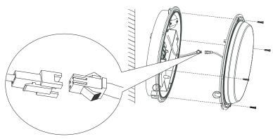
**6**: Buckle the frame back and fix it by proper tools.
