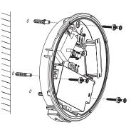
**4**: **a**. Connect the plugs between the battery and driver if with emergency function. **b**. Choose the power with DIP switch if it's the wattage changeable version (12 inch only). **c**. Connect the AC wires to the block.
