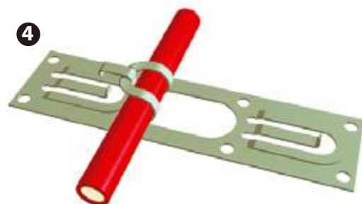
Fixing of the heating cable on the ECfast fitting band.
