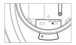
8 Wattage Selection: Slide the switch to the selected wattage. The sequence is as below.
