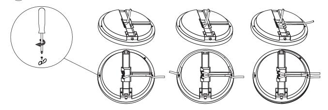
**5** Secure the bracket to the ceiling.
