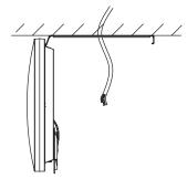
7 Connect the AC mains switched live, permanent live and neutral to the terminal block.
