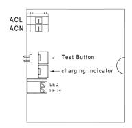
**Reset Plug**: the reset plug needs to be always inserted during operation. Remove the plug on emergency mode, then insert the system can be reset.
