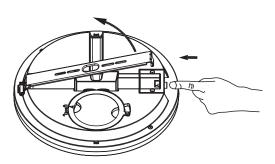
Twist the power cover of the anticlockwise and pull to remove it.
