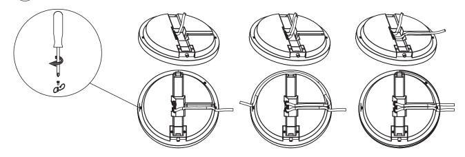
5 Secure the bracket to the ceiling.
