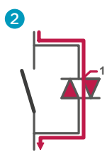
Start: conduction through the semiconductor.
