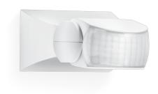
Targeted detection and attractive price. Infrared motion detector IS 1, for indoors and out, ideal for targeted coverage of small areas, 120° angle of coverage, reach up to 10 m, selectable time and twilight threshold, sensor turns through 30° and tilts through 180° for exact adjustment of the detection zone.
