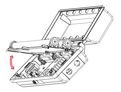
Gaining access to the terminals is achieved by rotating assembly of the reflector.
