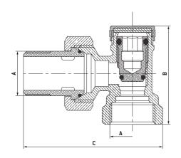
• Female angle lockshield valve with connection for iron pipes
