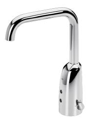
Touchless washbasin faucet with a temperature adjustment handle. Battery-operated 6 V. Length of spout 170 mm. The faucet is equipped with litter filters, non-return valves and Autofocus sensor which enables installation without adjustments. The adjustment values can be changed according to the conditions in the place of use with pre-programmed parameters. The impulsecontrolled solenoid valve gives the battery a long operating life. Flow controller (6 l/min) enables low water consumption.
