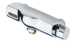
Touchless shower faucet that reacts quickly and precisely to the changes of water pressure and keeps the water temperature as selected. Suited to places where there are several water outlets and the network always contains plenty of hot water. Battery-operated 6 V. The temperature adjustment handle is equipped with a temperature limiter which can be bypassed by pushing a button. The faucet is equipped with litter filters and non-return valves.
