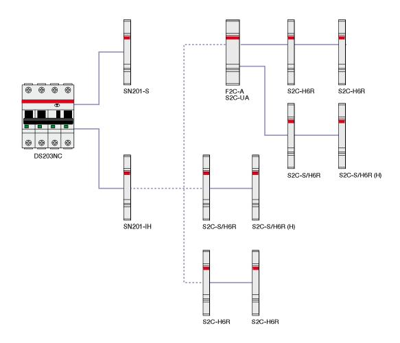
SN201-IH = coupling interface / auxiliary contact
