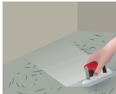
Filling grooves and irregularities on the substrate Surface
