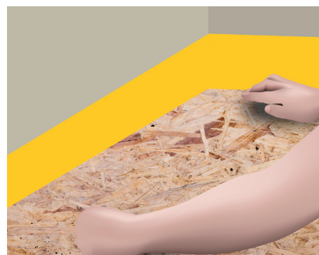
Installation of the edge strip/ EPS board cutting
