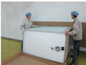
The modules with no frame: Two persons pull the peripheral board up and then place the board between the package and the upholder to protect the modules.
