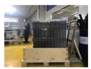
9. Note: The Modules must be stacked trimly, if moving the modules horizontally, please use the packing belt to fix the modules, otherwise the Modules may lean or even fall down during the transportation. Lift the Modules by the frame only; when carrying and lifting the Modules be careful not to twist the Modules.
