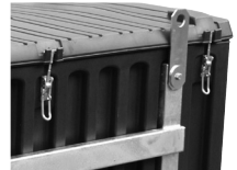
Figure 4.2.3.2: Crane lugs pivoted up
