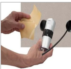
3. Open the bag OKT and remove the adhesive internal protection film
