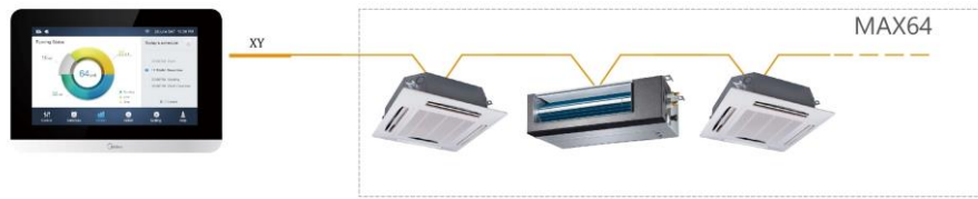
Figure 7(b) Connecting the centralized controller to the IDU (the first generation of AC/DC IDU)
