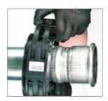
The press collar can only be removed from the press joint if both intermediate jaws (ZB 321 and ZB 322) were used.
