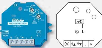
**300W power MOSFET.** Only 0.6 watt standby loss. With adjustable minimum brightness and dimming speed. With switching operation for light alarm clocks, children's rooms and snooze function. Also for dimmable energy saving lamps.
