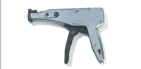
2) On the cable tie tension tool (P/N CM00000006) set the tension to 250N (position 6 on the index);
