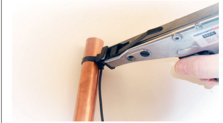
3) Use the tool to tighten and then cut the cable tie;
