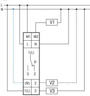
If (N) is connected, the zero passage switching is active.
