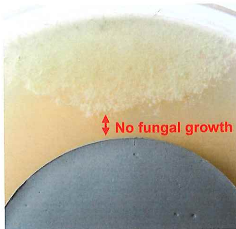
Photo 2: Material Zwaluw Acryl Ducting Seal (colour grey) : No growth of the test fungi could be detected directly around the material.
