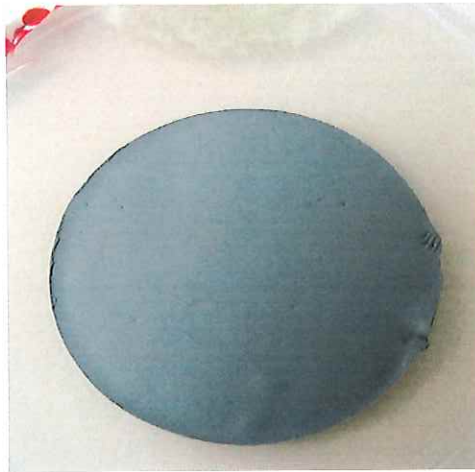
Photo 1: Material Zwaluw Acryl Ducting Seal (colour grey) : fungal growth was not visible to the naked eye
