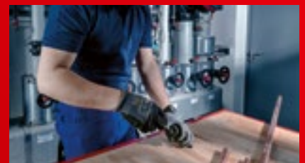
Retractable pipe deburrer—No extra tool needed to prepare a perfect connection
