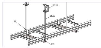
The cable ladder is attached to gate support PRT with bracket KK. Gate support PRT is attached to threaded rod GT-10 with nuts MU M10.
