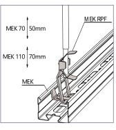
The RPF suspension is quick to install and adjustable. The threaded rod is attached to the ceiling with either ceiling bracket RTF-10 or another, appropriate method, such as an expansion bolt.
