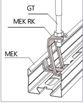
MEK RK is attached to threaded rod GT-10 with two M10 nuts. The threaded rod is attached to the ceiling with either ceiling bracket RTF-10 or another, appropriate method, such as an expansion bolt. Once the ceiling suspension is in place, the lighting support rail can be installed to the intermediate support.
