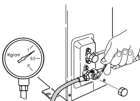
**EG** Turn on the unit's operating switch and start cooling operation. When the low-pressure gauge reading falls to 1 to 0,5 kg/cm<sup>2</sup>, fully close the wide tube stern and then quickly turn off the unit.
