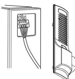
**EG** Remove the side cover (or access panel) then connect the power line and interconnecting wires to outdoor unit on the terminal strip and secure them with clamps.
