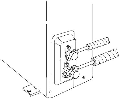
**E** Remove the valve manifold. At that time, PUMP DOWN has been completed and all refrigerant gas will have been collected in the outdoor unit.
