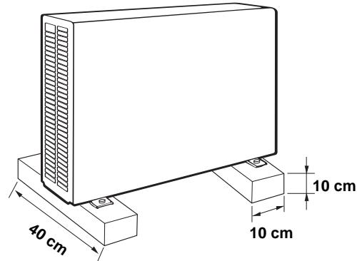
Provide a solid base for outdoor unit raised from the ground level. Fix unit to base using 4 anchor bolts.
