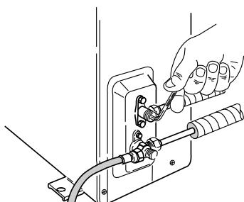
**EG** With vacuum pump still running close the low pressure knob on valve manifold. Then stop vacuum pump. Using an hexagonal key open the service valve on small tube, then close it after 10 seconds. Check tightness of all joints using liquid soap.
