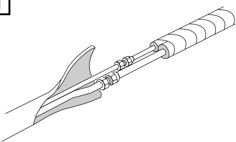
**EG** Insulate tubes leaving connections uncovered for leak test.
