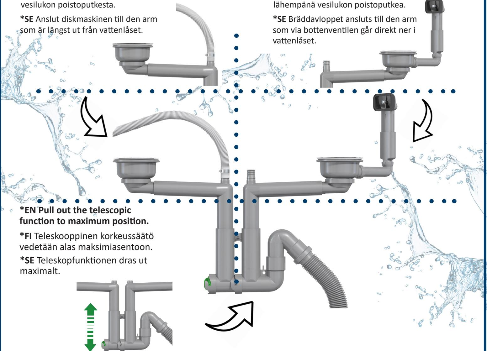
**\*EN Pull out the telescopic function to maximum position.**
