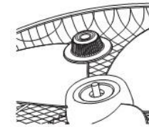
Fig. 2 Spinner tighten anti-clockwise
