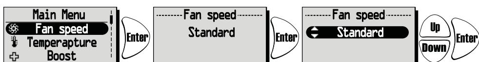
For HERU®EC, standard speed/mode during normal operation.
