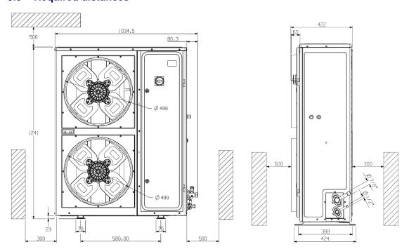
Figure 21: Fixing dimensions and distances
