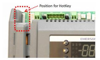
Figure 14: Location of "Hot Key" plug connection
