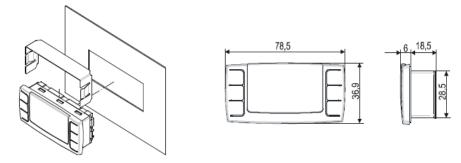
Figure 10: Remote display front panel mounting
