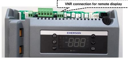
Figure 11: VNR connection for the remote display
