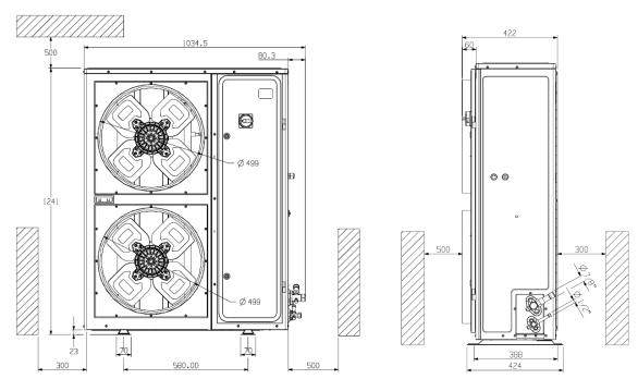
Figure 16: Dimensions of ZXDI condensing units (all models)
