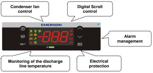
Figure 7: XCM25D controller functionality overview
