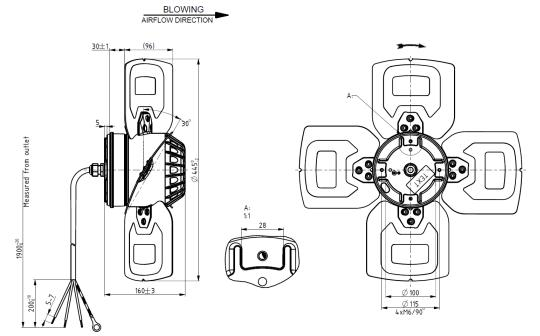
Figure 2: Fan details and dimensions
