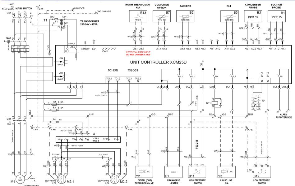
Figure 24: Wiring diagram - 3-Phase motor
