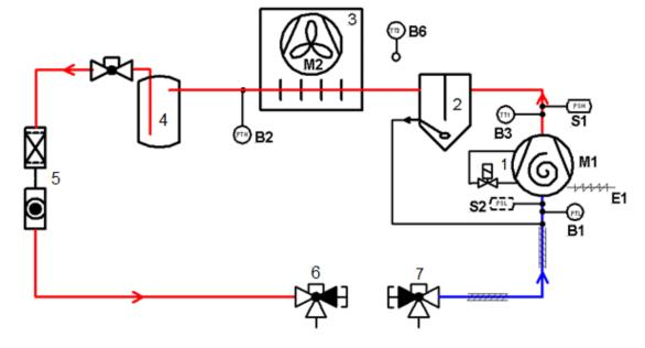
Figure 5: P&I diagram for ZXDI units
