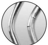
Beside picture shows two ground rods subjected to the same pressure load test.
